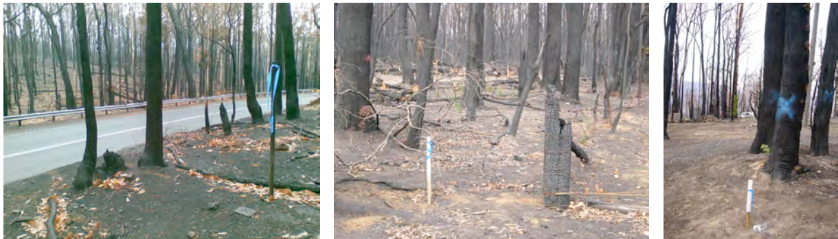
Figure 2. (L-R) Permanent mark, reference mark and timber peg found and staked by volunteer surveyors.
