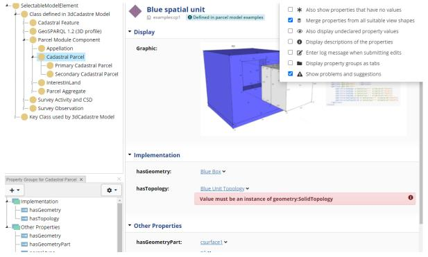
Figure 11: Example of a test data validation report in the SOP User Interface
