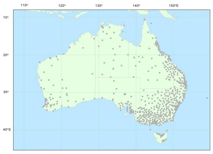
Figure 2. The location of Continuously Operating Reference Stations in Australia as at January 2019.
