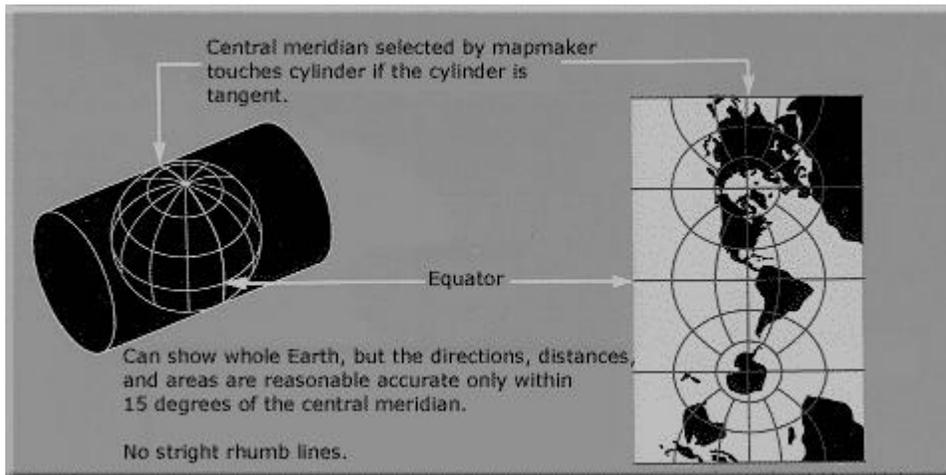
**Used** by USGS for many quadrangle maps at scales from 1:24,000 to 1:250,000; such maps can be joined at their edges only if they are in the same zone with one central meridian. Also used for mapping large areas that are mainly north-south in extent.
