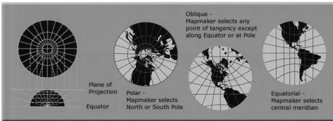
**Used** along with the Mercator by some navigators to find the shortest path between two points. Used in seismic work because seismic waves tend to travel along great circles.
