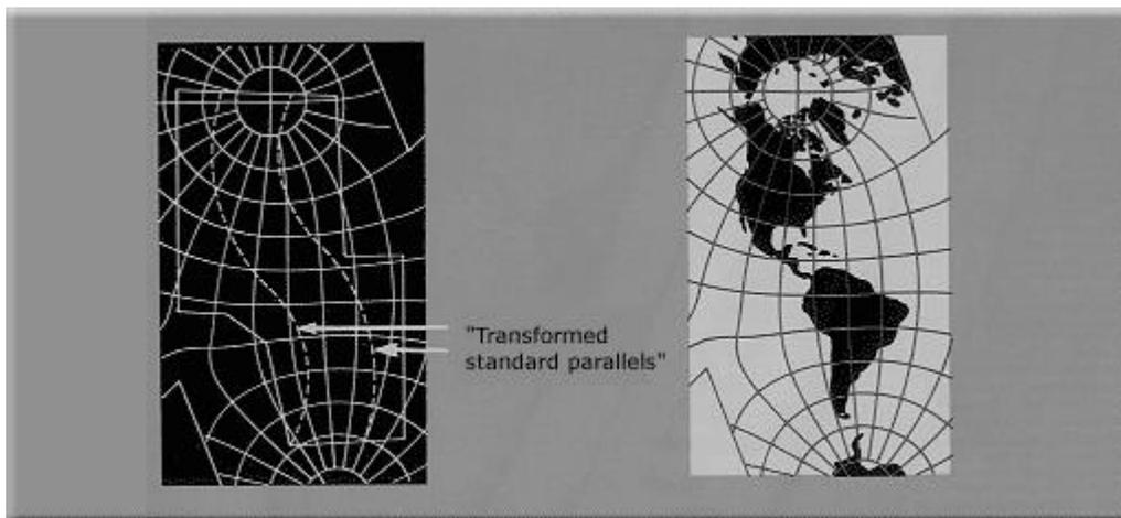
This "tailor-made" projection is **used** to show one or both of the American continents. Outlines in the projection diagram represent areas shown on USGS Basement and Tectonic Maps of North America.
