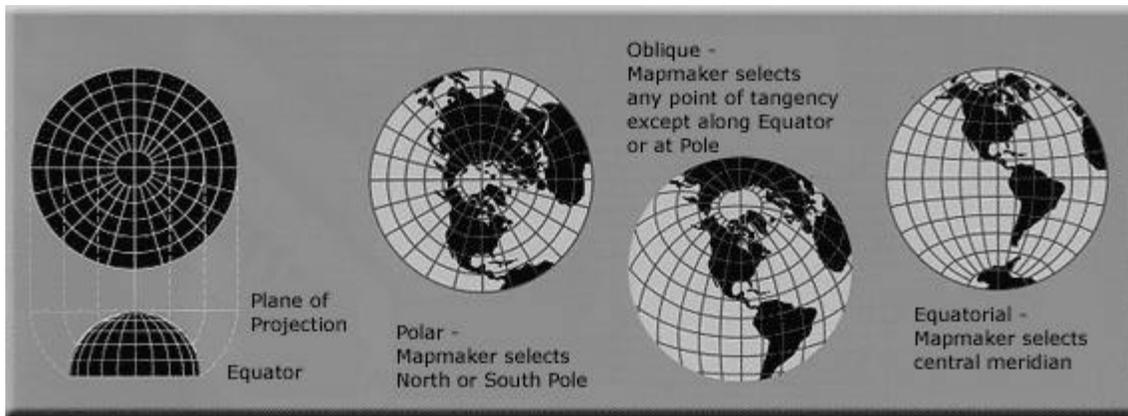
Used by USGS in the *National Atlas of the United States of America*<sup>TM</sup> and for large-scale mapping of Micronesia. Useful for showing airline distances from center point of projection. Useful for seismic and radio work. Oblique aspect used for atlas maps of continents and world maps for radio and aviation use. Polar aspect used for world maps, maps of polar hemispheres, and United Nations emblem.
