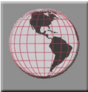
**Globe**, as represented by Orthographic projection—equatorial aspect.
