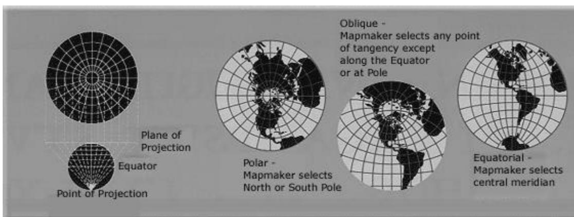
**Used** by the USGS for maps of Antarctica and American Geographical Society for Arctic and Antarctic maps. May be used to map large continent-sized areas of similar extent in all directions. Used in geophysics to solve spherical geometry problems. Polar aspects used for topographic maps and charts for navigating in latitudes above 80°.
