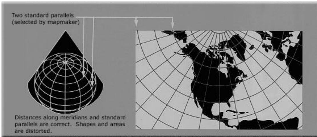
**Used** in atlases to show areas in the middle latitudes. Good for showing regions within a few degrees of latitude and lying on one side of the Equator. (One example, the Kavraisky No. 4, is an Equidistant Conic projection in which standard parallels are chosen to minimize overall error.)
